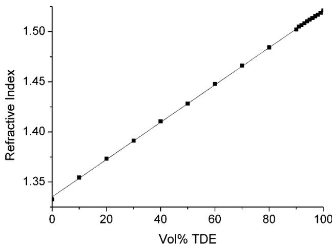
Fig. 3. TDE (2,2'-thiodiethanol) is miscible with water in any proportion. The refractive index of the solution can be precisely tuned to any value between 1.333 (water) and 1.521. The latter is even slightly larger than that of immersion oil.
