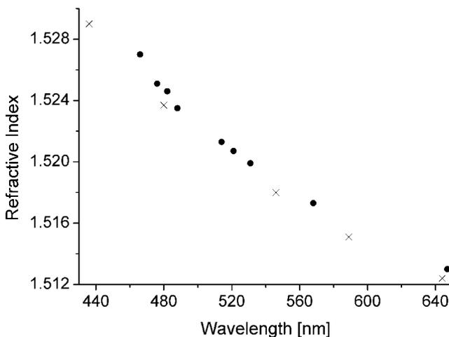
Fig. A1. The dispersion of TDE (dot) is close to the dispersion of standard immersion oil (Leica Microsystems) (cross). This avoids the chromatic aberrations otherwise introduced by the mounting medium.
