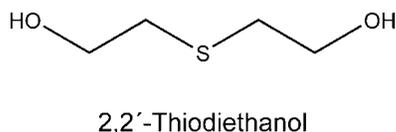
Fig. 2. TDE (2,2'-thiodiethanol) is a nontoxic glycol derivative which, owing to the sulfur atom, exhibits a large polarizability and hence a high refractive index. It is soluble in water at any concentration.
