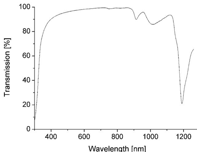
Fig. A3. The transmission spectrum of TDE (10 mm thickness) shows minimal absorption over the entire visible and near infrared range. For a microscope sample of  $100 \mu\text{m}$  thickness, the transmission in the 360–1,100 nm spectral range is  $>99\%$ .
