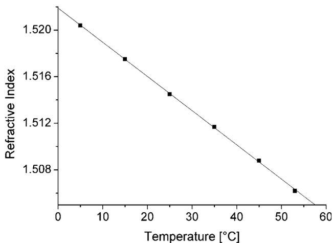
Fig. A2. The temperature dependence of the refractive index of TDE ( $3 \times 10^{-4}/^{\circ}\text{C}$ ) is slightly less than that of the immersion oil ( $3.8 \times 10^{-4}/^{\circ}\text{C}$ ).
