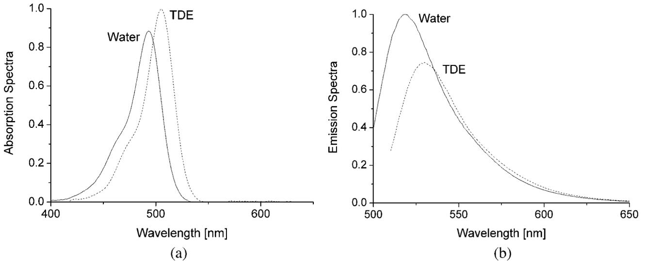
Fig. 7. Comparison of the absorption and emission spectra of Oregon Green 488 in water and in 97% TDE. The spectra are red shifted by 12 nm.
