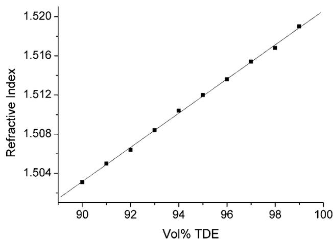
Fig. 4. TDE allows a precise setting of the refractive index by adjusting the water content. For use with an oil immersion lens, a TDE concentration of 97% in water was employed.
