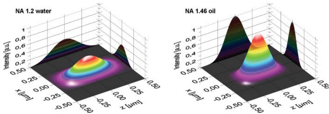
Fig. 1. Surface plots of an axial section ( $xz$ ) of the main maximum of the PSF of a confocal microscope for a water immersion lens with  $NA = 1.2$  (left) and an oil immersion lens with  $NA = 1.46$  (right); excitation, 488 nm; emission, 525 nm. The PSF of the oil immersion lens is narrower by 30% along the  $z$ -axis. Additionally, the 30% larger collection and excitation efficiency results in a doubled peak intensity.
